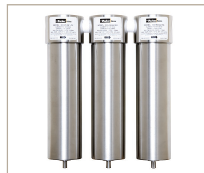
Fig. 4. The final stage of filtration, in 304 stainless steel, removes all viable organisms with an efficiency rating of 99.9999+% at 0.01 micron (5 log reduction).
